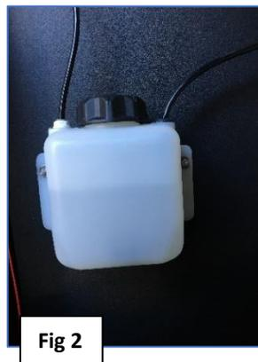
2. Mount the water reservoir **below** the system enclosure by about 12-16 inches (see Fig 2). Secure the water reservoir with the screws to the bulkhead.
