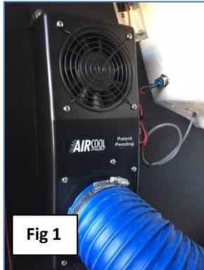
1. Locate a suitable place to mount the system enclosure. The enclosure should be mounted vertically with the fan assembly up and the vent down (see Fig1). Using the four holes in the corner of the base plate, screw the system down using large flat washers to secure the enclosure. Please note there is a 3/8" drain in the bottom of the enclosure which allows for a tube to be installed to direct the water drainage if necessary.
