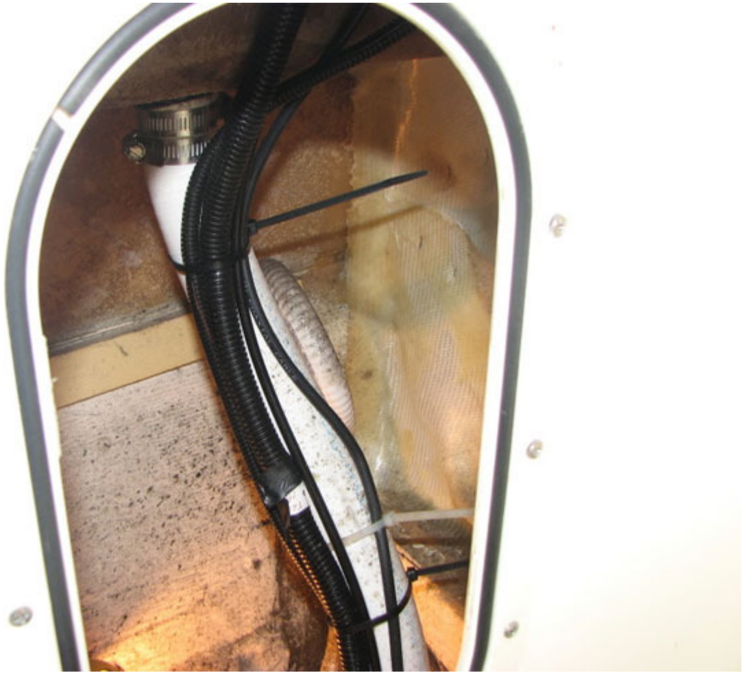
Pict #11: Misting Tube (2nd from Right) running up the Port side Hardtop Leg.
